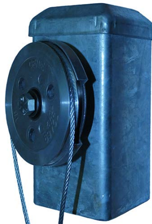
4. Winch cable inserted into pulley groove
