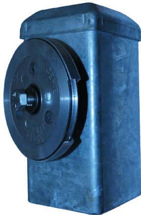
3. Pulley wheel retaining bolt loosened to allow winch cable routing
